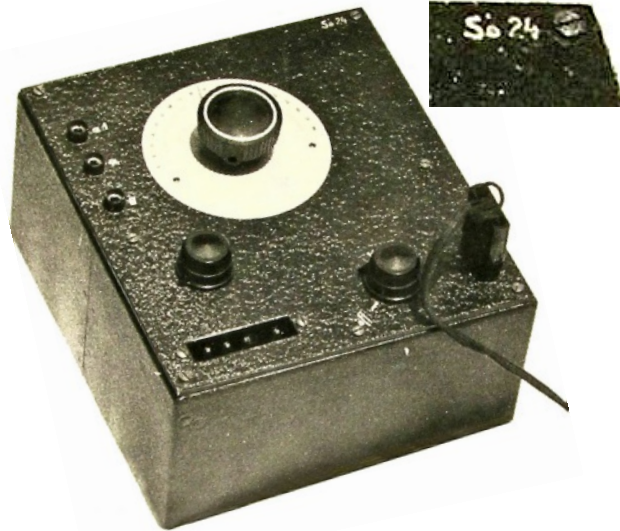
E 88 receiver, part of an SE 88/5. Serial number in enlarged cutout was So 24.
