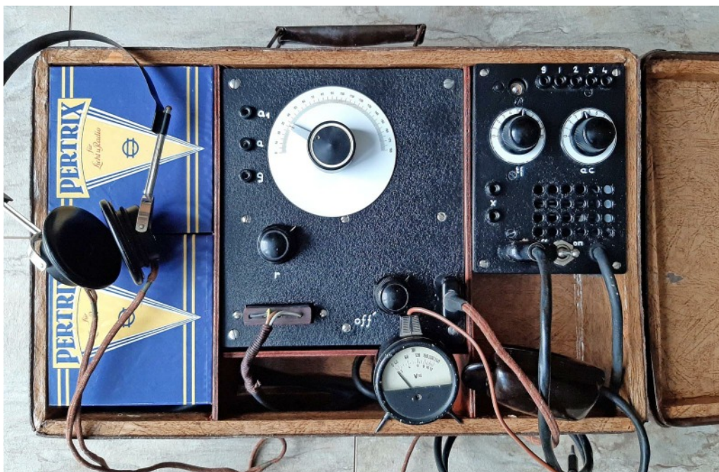
SE 88/5 replica from the collection of DJ5RE, often used for radio contacts in the 40m amateur radio band.
