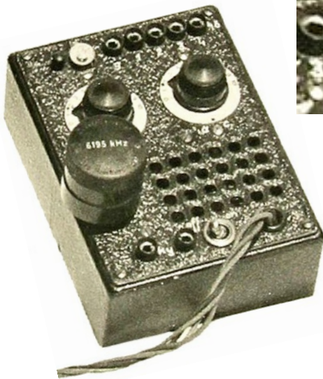
Transmitter unit of the SE 88/5 (S 88/5) with serial number 46 in enlarged cutout.
