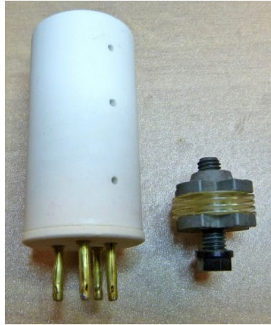
Hirschmann ceramic coil (left) Siemens powdered iron core coil (right).
